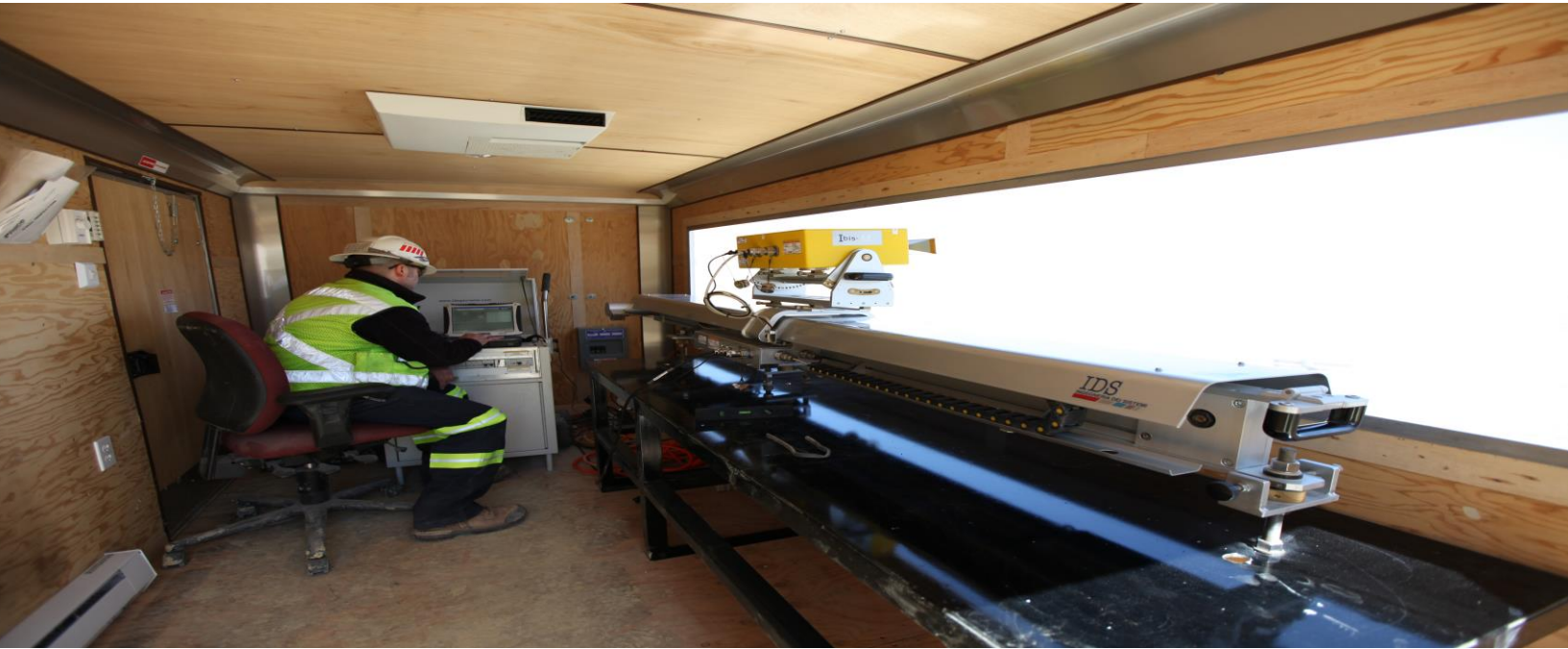
Above: Slope monitoring with Kennecott's IBIS radar system
